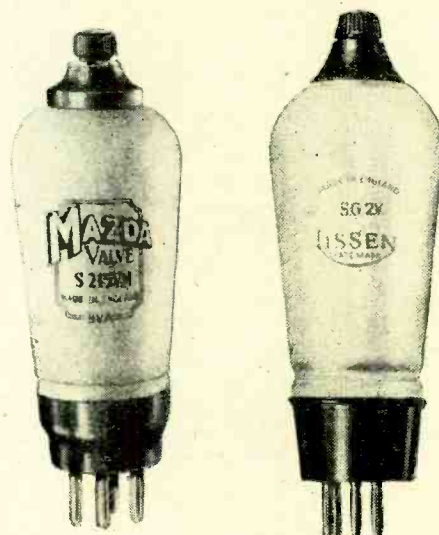
Mazda 2-volt battery variable-mu, the S 215VM, and (right) the Lissen 2-volt battery type the SG2V.
