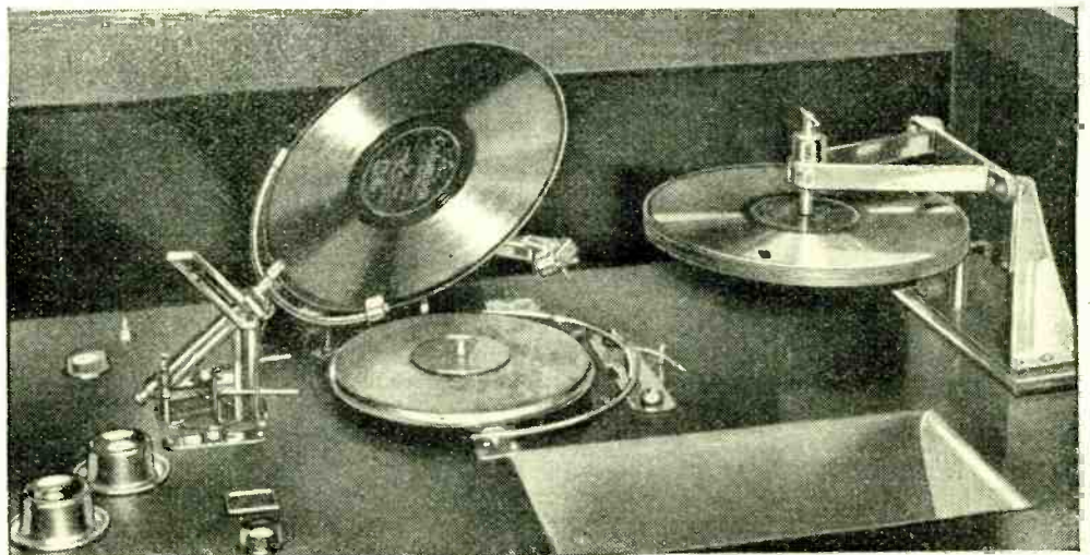
The Gilbert record-changer turns over each record and plays both sides.
