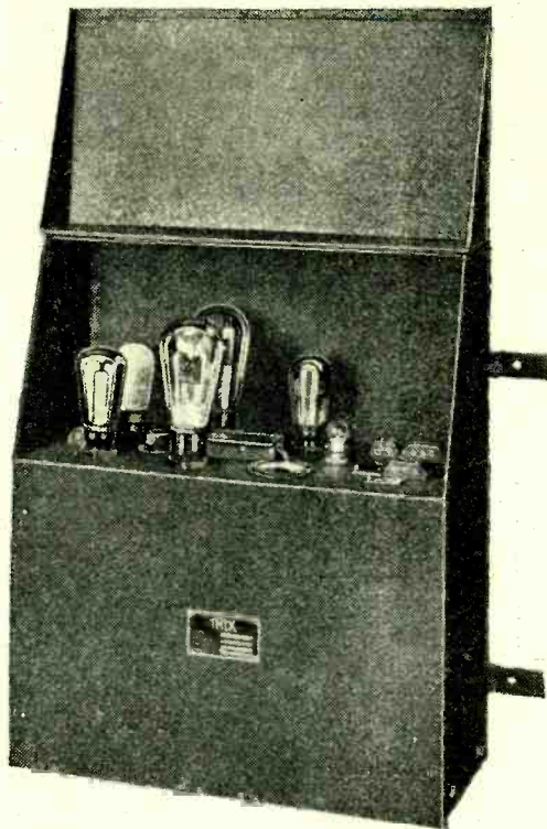
In the upper compartment are housed the four amplifying valves, the mains rectifier and the tone control.
